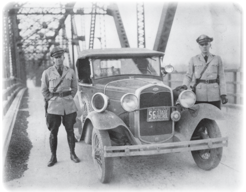
Tprs. M. Dace and J.A. Tandy (right) stand next to a 1932 Ford Model A. Notice the new warning light on the right fender which aided troopers in stopping motorists at night.
