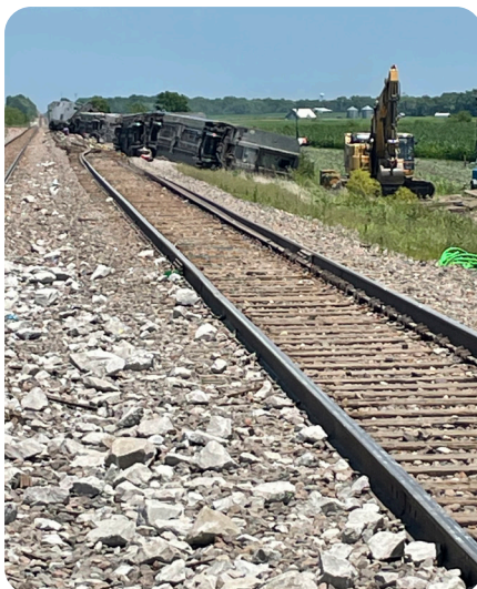
This photo shows derailed Amtrak cars and damaged track after the train/dump truck crash.
